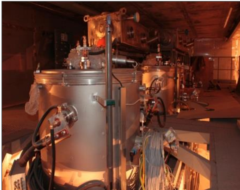
System for fuel pellets sintering, MOX fuel fabrication
