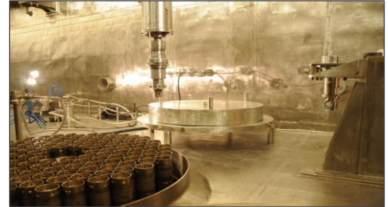
SNF reloading into a 'dry' storage facility at MCC
